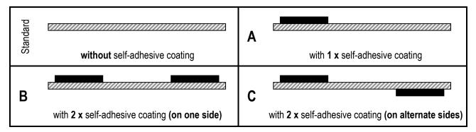
Self-adhesive coating up to 150 mm foil width 20 x 1 mm butyl rubber up to 200 mm foil width 40 x 1 mm butyl rubber
