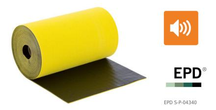
FONODAN BJ is a two layer product made of a self-adhesive high density bitumen membrane thermally bonded to a cross-linked polyethylene. FONODAN BJ acoustically works providing the acoustic mass of the tube body and removing resonant frequencies.
